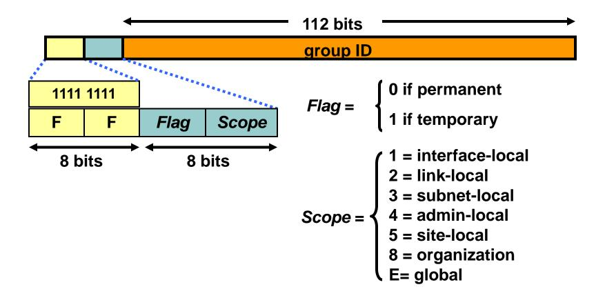
Multicast is used in the context of one-to-many. A multicast scope is new in IPv6.
