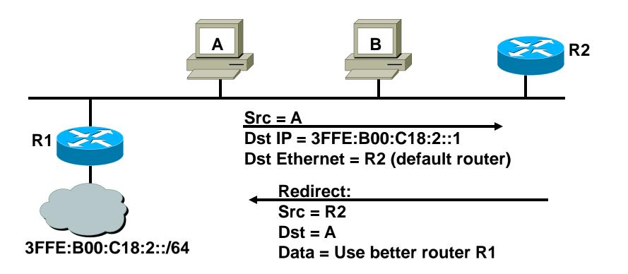
Routers use ICMPv6 Type 137 redirection messages to inform nodes on the link that a better router exists on the link to forward packets.
